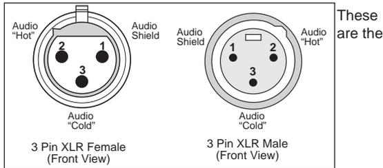
standard pinouts for balanced leads using 3 pin XLR plugs and sockets. Audio "Hot" is the in-phase connection, whilst Audio "Cold" is the out-of-phase connection. Should an unbalanced lead be required, one of the audio pins must be referenced to ground ie. Pin 3 and 1 are connected together OR pins 2 and 1 are connected together. The last pin is used for the audio signal.
