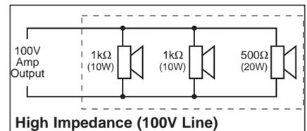
$$\frac{1}{\frac{1}{1k\Omega} + \frac{1}{1k\Omega} + \frac{1}{500\Omega}} = 250\Omega (40W)$$
