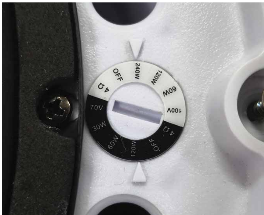
The dial control is to set input mode because this is a passive subwoofer, not an active one. It has no built-in amplifier. It has five positions. One is off.
