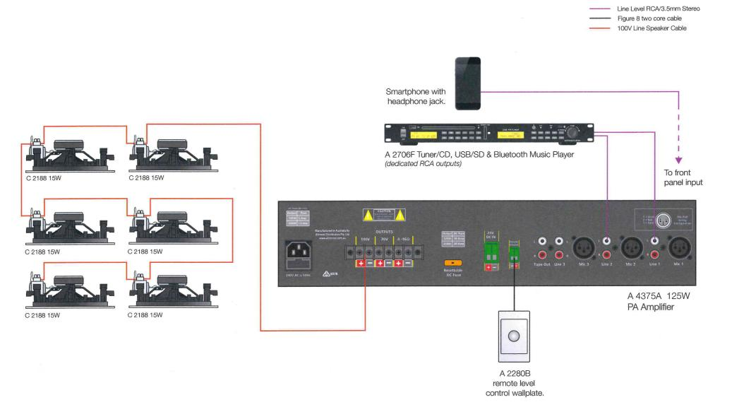
If Bluetooth connectivity is required, smartphone may be replaced with a Bluetooth streaming adaptor such as Altronics A 1109
