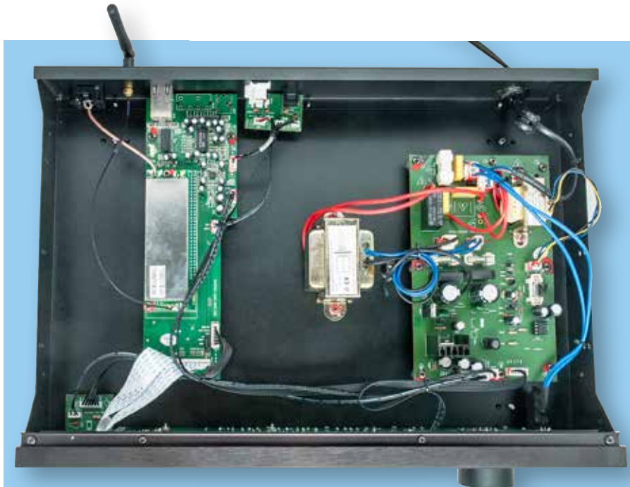
Inside the A2696 – the Venice 6.2 module is the shiny metal box on the left and is mounted on a PCB along with some support circuitry. The large PCB on the right is the power supply while another PCB at the front holds the front panel display and controls. The Venice module does all the work and everything else is just there to support the module.
