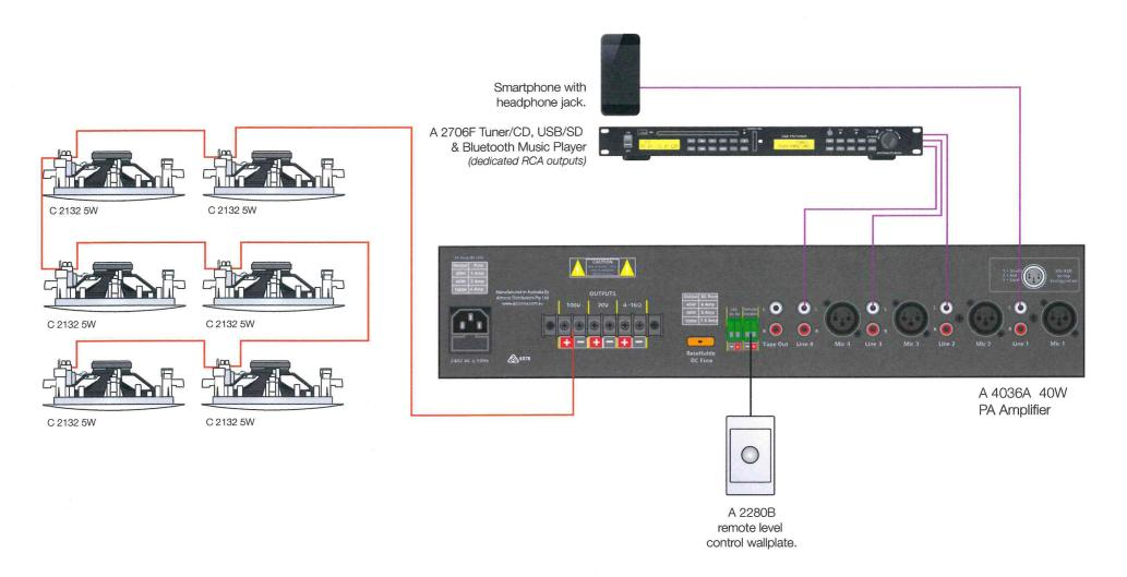
If Bluetooth connectivity is required, smartphone may be replaced with a Bluetooth streaming adaptor such as Altronics A 1109
