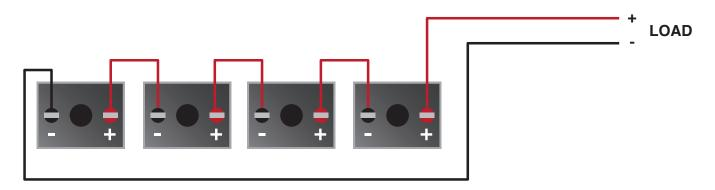
Note: When using LiFePO4 batteries in circuits, NEVER mix brands, capacities or voltages. Always use identical batteries in your circuit (ie: same brand/model, same amp hour (Ah) rating, same voltage).
