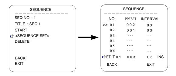
Move the cursor to EDIT and press IRIS ON to enter edition mode. Move the joystick rightward and leftward to select item.
