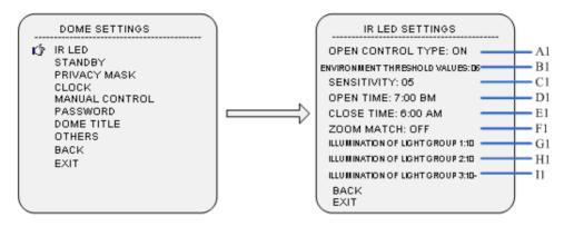
Move the cursor to "IR LED", and press iris open to submenu.
