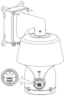
4. Attach the drill positioning paste to the wall, and drill according to the paste, and install expansion bolts.
