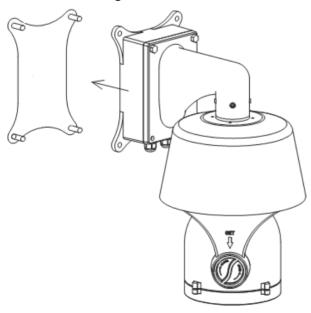
6. Remove two screws from the power box, and open it.
