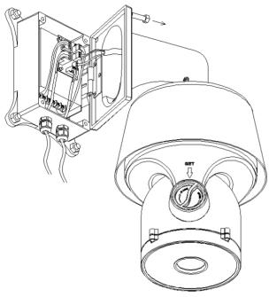
7. close power box, tighten the bracket to the power box. Double check if there is joint gaps, if necessary, apply water-proof glue.
