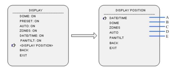
Move cursor to DISPLAY POSITION and press "Iris on" to enter submenu of DISPLAY POSITION
