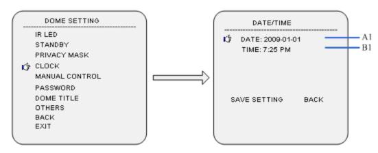
Move cursor to CLOCK and press "Iris on" to enter the submenu of CLOCK.
