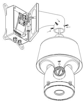
3. unscrew the cover with the mark "SET", set communication protocol and addresses. Screw up again with care to avoid water.
