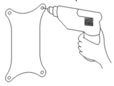
5. Install the dome body together with bracket and power box to the expansion bolts, and tighten with screws.
