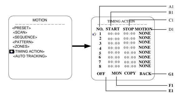
TIMING ACTION: The user could set up the required functions during the designated time periods. These functions include presets, cruising track, pattern tours and scanning.
