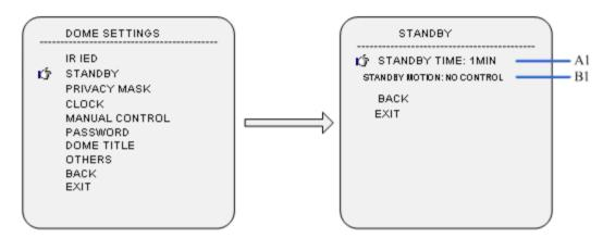
Move cursor to STANDBY SETTINGS and press "Iris on" to submenu of STANDBY SETTINGS.
