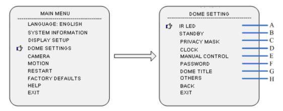
Call upon preset position 95 to enter the setting interface of the OSD menu and move joystick to "DOME" press "Iris on" enter submenu of "DOME".
