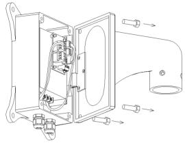
2. Thread cables across the bracket and connect them to the circuit board in the power box.
