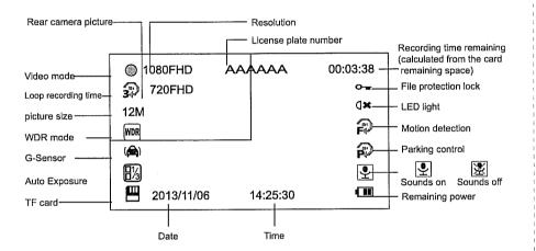
Note: Only connect with rear camera the LCD display will show 720P and picture in picture( without rear camera no display)
