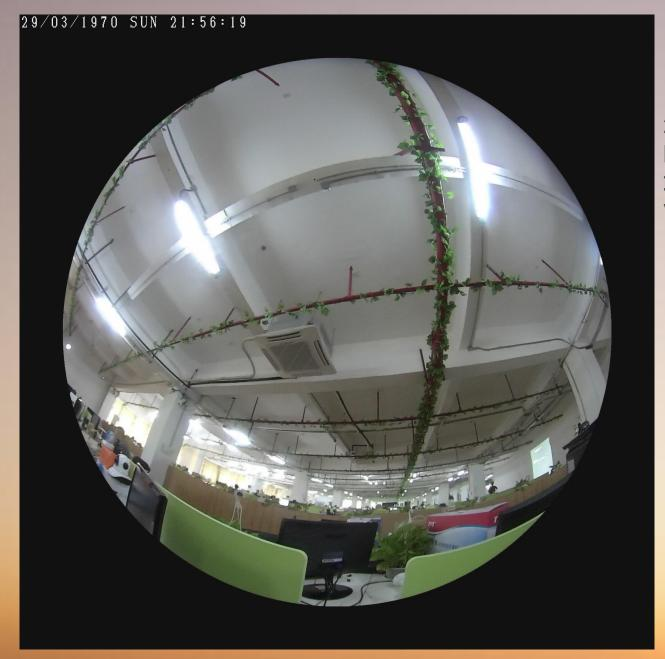
鱼眼IPC F300, S600, S1200输出的图像为180度视角的圆形图像, 图像纠正还有VR功能需要在客户端软件VMS, 手机app上, 或者是后端NVR上才能实现 The output image will be 180 degree. VR function will be worked in Client VMS, app and NVR. 3
