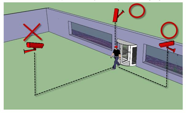
2. The detected size of the target should be between 1/500~1/10 on the screen.
