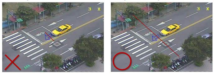
4. The virtual detection line should be drawn vertically to the moving target.
