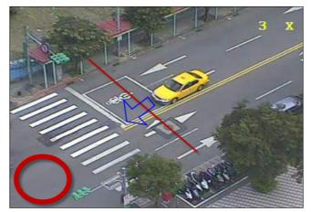
5. The target should be able to cross the virtual detection line completely in order for the counting process to be completed.
