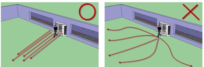
8. Allow the front and back of the virtual detection line to be clear. Prevent setting the line at a place near many constant moving objects.
