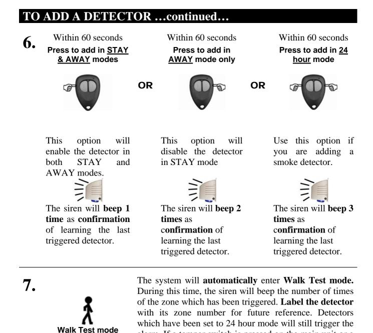
**NOTE:** Refer to (5) If you trigger a detector that is already learnt in you will hear one low tone beep, simply trigger the correct detector until you hear the siren give the normal zone confirmation beeps. You need to do step (6) after the correct detector has been acknowledged, as it will keep accepting any unlearnt detector until step (6) is done or it times out (60 seconds).
