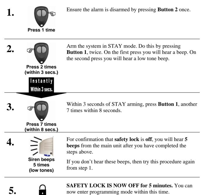
**NOTE:** If you cannot enter programming mode, this is because safety lock is on. If you cannot turn off safety lock, this would mean safety lock is already off.
