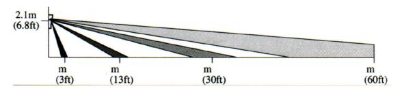
Figure 9 – side view, detection pattern in optimal temperature environment
