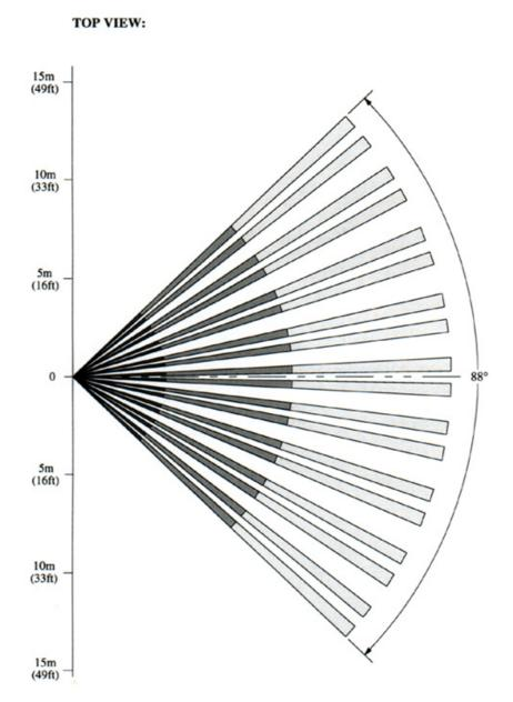
Figure 10 – detection pattern in the optimal temperature environment
