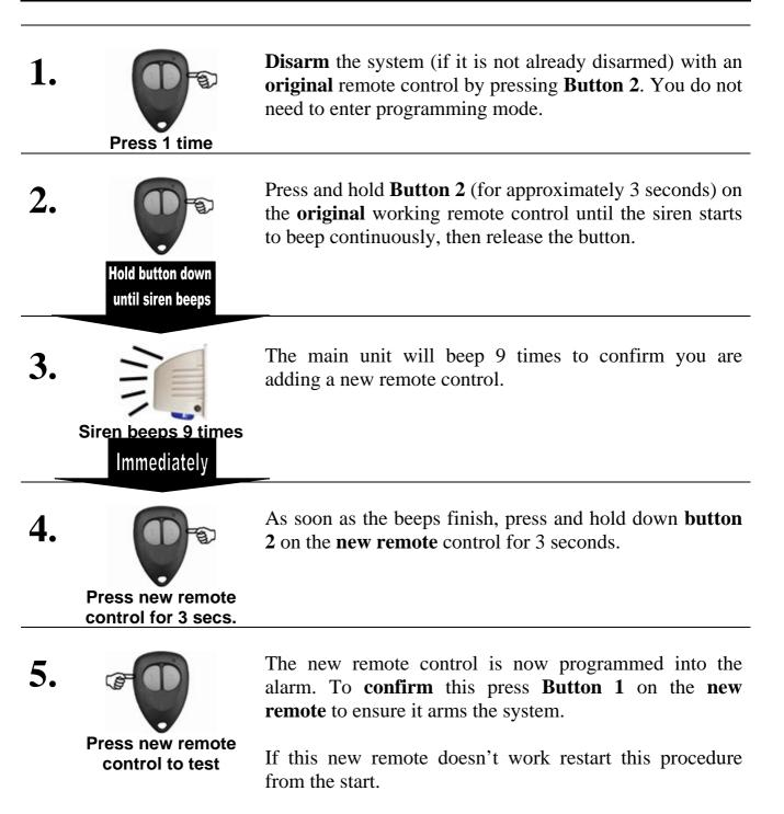
Your *Watchguard Home Alarm System* can only store a maximum of **SEVEN** (7) remotes in its memory. If you learn in an 8th remote, the 1st remote control will be erased. If you loose a remote control, or have one stolen, simply repeat the procedure above with your remaining remotes at least 10 times. This will ensure that you have erased the lost remote from the memory of your *Watchguard Home Alarm System*.
