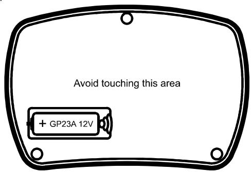
The battery should only be replaced with a high quality battery identical to, or equivalent to an Alkaline GP23A or MN21 12V (10mm diameter x 28mm length). Replacement batteries are available directly from Peak Electronic Design Limited and many good electronic/automotive outlets.
