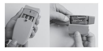
Replace the 3 x 1.5V AA (R6) batteries for the transmitter and 1 x 9V (6F22) battery for the receiver.
