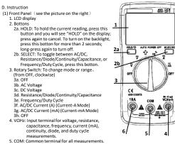
6. 10A: Input terminal for current (A) measurements.
