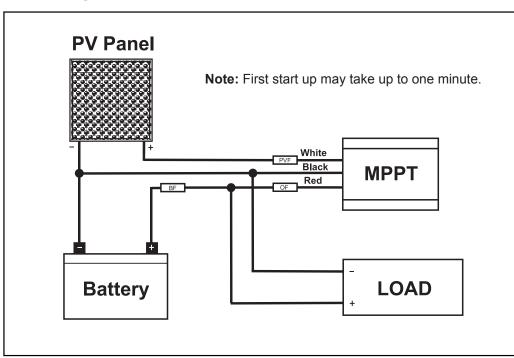
Note: This unit can be to used to directly power (without a battery) a 12VDC motor or pump of up to 100W.
