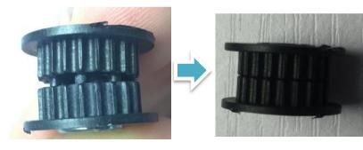
The 2 sides of idle pulley is snapping fitted with 3 pillars into slots. Pay attention to the orientation to ensure they match EXACTLY.
