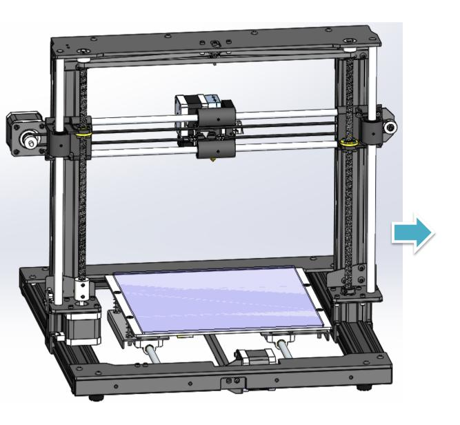
Use clips to fix the glass on the heating plate
