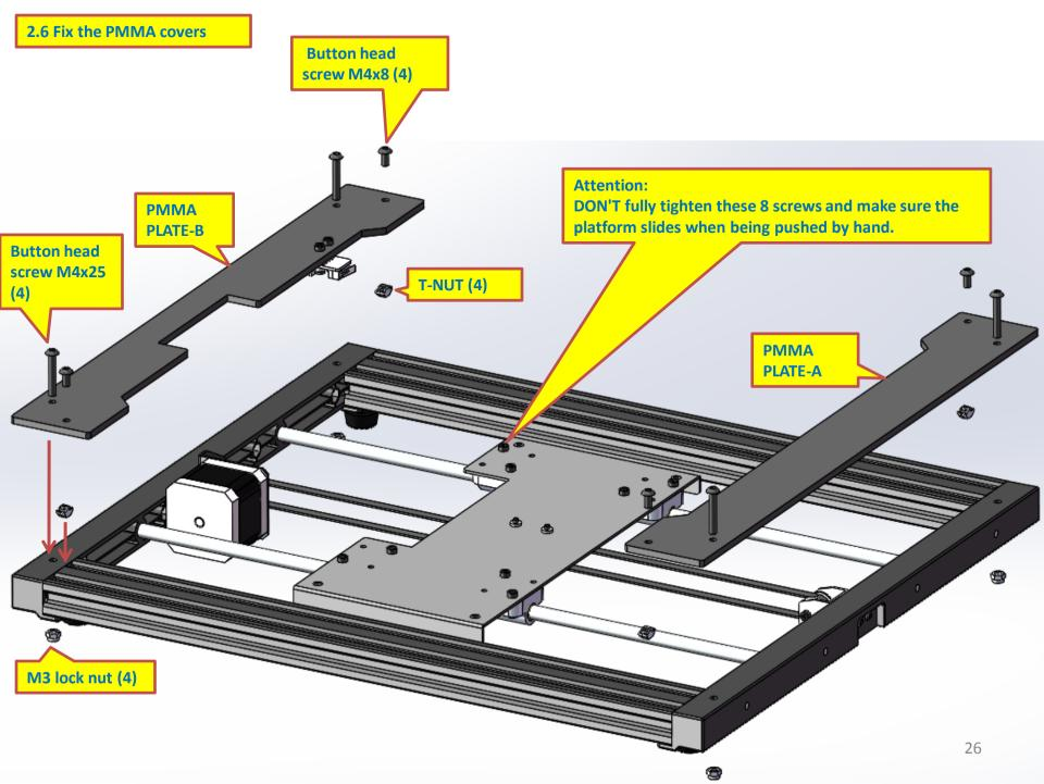
Assembly of Y motion system is complete.
