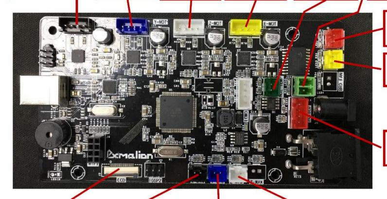
Nozzle cooler fan marking: NOZ-FAN socket: XH-2P red
