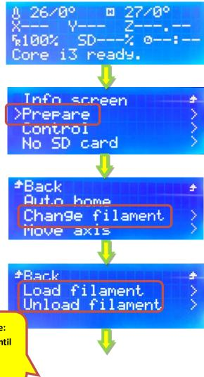
Nozzle temperature / set temperature: load / unload filament cannot start until nozzle temperature reaches the set value.
