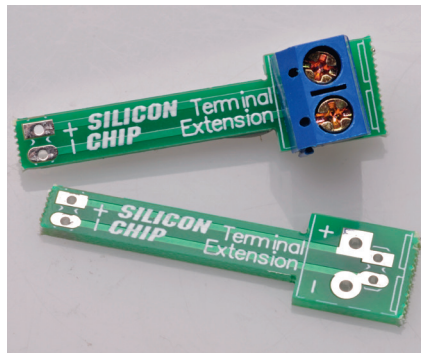
Photographs: The Opto-Isolated Relay mounted inside a UB3 Jiffy box with the mains power plug and power socket wired up. Note the terminal extension boards, as shown above, are wired positive (+) to positive. These are optional attachments to make connecting your control module easier.
