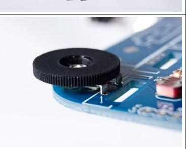
Now insert the first wheel into the PCB as shown.
