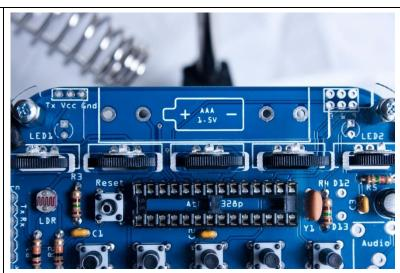
Then you can solder the pins on all the thumbwheels.
