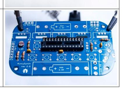
Now add the ceramic oscillator, Y1. Again, there's no polarity, so it can go either way. It helps to have some method of holding it vertical while you solder. Here I've used one of the clips on the helping hand to support it while I solder.
