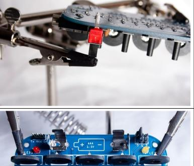
If you'll be using the preinstalled software, put the jumper in place in position 3 as shown. You also have the option of using digital pin 6 or 9 for the audio output if you're using other software. **Note: don't forget the jumper, or you won't get any sound. It's easy to forget.**
