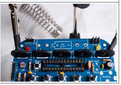
Now we'll add the audio jack as shown. These pins are bigger than on any previous components, so it will take more solder to make a good joint. Use plenty so the jack will be firmly attached to the PCB.
