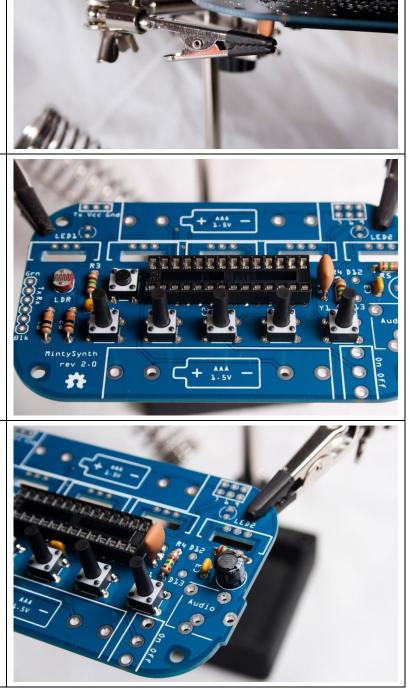
Now we're ready for the five thumbwheels. To prepare them, bend the single unused pin upward as shown in the photo. It should still be angled outward just slightly (maybe 5-10 degrees). This pin will engage in the underside of the acrylic cover plate, holding each wheel securely.
