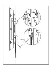
Please install the ribbon by lateral. Pull down the ribbon to lock, Pull up the ribbon to unlock.
