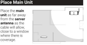
Ideally it should be placed with at least one wall between the donor and server antennas. If the patch antenna cable is too short, it may be extended.
