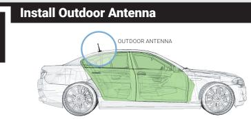
Mount your **Outdoor Antenna** on the exterior of the vehicle, towards the rear, according to its design, and the type of vehicle it's being used with. Make sure you consider the cable connection to the **CEL-FI GO** unit with your location choice.
