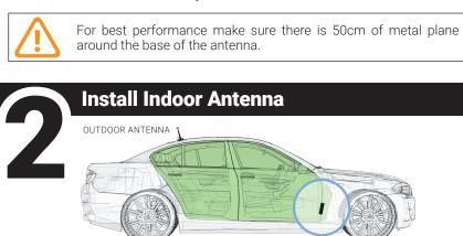
Install **Indoor Antenna** in the cab, towards the front, where coverage is needed. Ideally, there should be substantial material, like the metal of the roof, between the **Outdoor** and **Indoor Antennas**, to improve isolation.
