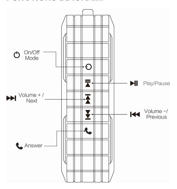
Modes: Bluetooth and FM Tuner. Long press is ON and OFF. Short press to switch modes.
