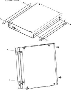
(2) DIN Rail: Fix DIN Rail clip to the UPS with two screws. Clip the assembled UPS unit onto the DIN Rail
