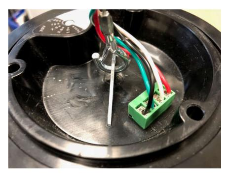
Secure wire hook to speaker hanging frame & terminate in/out speaker connections to plug.
