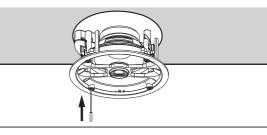
4. Lock the speaker by pressing the buttons located on the front face of the speaker and the dog leg will engage automatically.
