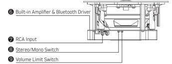
Limiter Enabled(50%): The volume will be limited. (max. output: 15W@8Ω) Limiter Disable(100%): The volume can be adjusted to the max. (max. output: 30W@8Ω)
