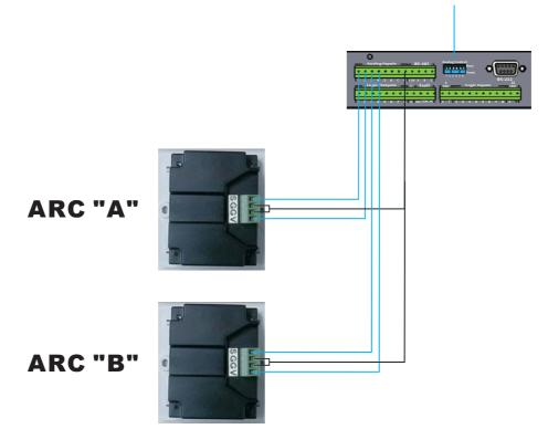
\*\* Each PDP can connects to 3 pieces of ARC (max.).
