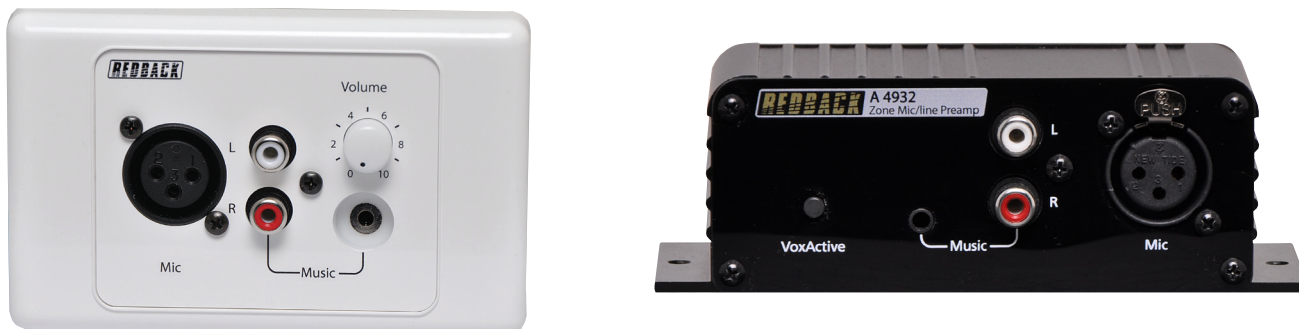
Fig 17. Front View of A 4931 Local Input Wall Plate and A 4932 Local Input Box
