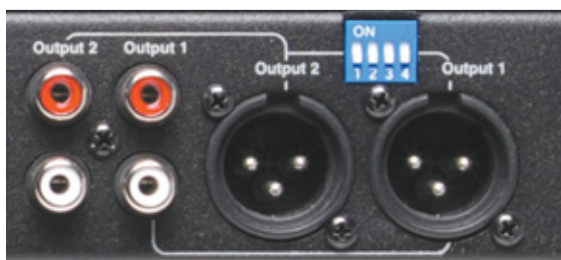
Figure 2: Rear panel DIP switches relating to outputs 1 and 2.
