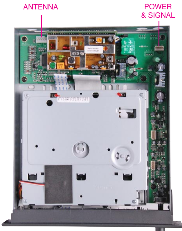
Figure 1: Location of antenna and power/signal headers.
