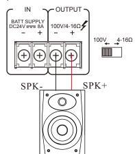
②When the 100V and 4-16Ω selector switch to 4-16Ω position, as shown below:
