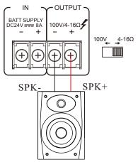
Constant pressure speaker: According to the rated power of the power amplifier, connect the constant power speaker
