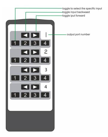
User can control the HDMI route of the matrix by using the IR remote.
