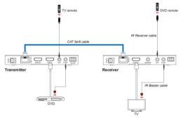
Note: When the angle between the IR receiver and the remote control is  $\pm$  45 °, the transmission distance is 0-5 metres; when the angle between the IR receiver and the remote control is  $\pm$  90 °, the transmission distance is 0-8 metres.
