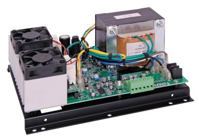
This module is designed for use in emergency evacuation systems and is powered by an external 24V DC source. It accepts a line level audio input and produces a 100V line output via a transformer. It also features short circuit, overload and thermal cutout protection, and is constructed on a steel chassis. Designed with reliability and robust performance in mind, it is the ideal audio power source for evacuation systems, or any application which requires a DC powered 100V line amplifier.
