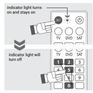
5. Check whether each function key of the remote control operates normally, if it does, it represents that the corresponding setting is successful; if some of the function keys don't operate normally, please repeat procedure 4 and input other code of the corresponding brand
