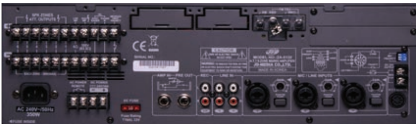
Rear panel shown with tuner connections fitted (See A 4344 & A 4346 below)
