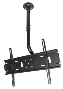
A heavy duty ceiling mount bracket suitable for mounting flat screens up to 75kg. The swivel mount allows 15° of vertical tilt adjustment and 130° of horizontal adjustment. The design enables adjustment to suit screens up to 800x500 VESA mount size. Mounting height from ceiling can be varied 100mm steps up to a max of 1.2m from ceiling (to edge of mounting arms.
