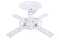
Designed to suit a wide variety of projector models, this ball joint bracket allows up to 30° of adjustment. The mounting surface sits between  $\approx$ 135 to 195mm (adjustable in 20mm steps) from the ceiling and may be removed from the upper bracket for adjusting projector settings. For high ceilings, extension poles allow projector mounting surface to be adjusted between  $\approx$ 440 to 760mm in 20mm steps. Includes two sets of mounting arms (140 & 180mm).
