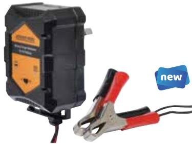
This 6V/12V battery charger maintainer provides 800mA charging current suitable for lead-gel and lead acid batteries, including maintenance free battery types. It is suitable for permanent connection to provide battery maintenance for disconnected batteries or for seldom used vehicles, boats, caravans etc. Provided with ring terminal connection and crocodile clips for simple connection to battery.
