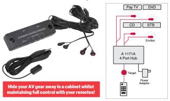
This complete infra red (IR) extender kit allows you to locate your AV equipment inside a cabinet, rack or cupboard. The signals are relayed to your equipment by the IR target, which can be located discretely under your TV (all target and emitter cables are 3m long). The four IR emitters transmit signals to your AV devices. Kit includes hub, one infra red target, two 'dual eye' infra red emitters and 5V DC power supply.
