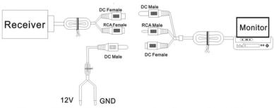
Connection of wireless receiver box and monitor
