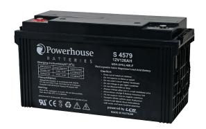
This 12V 126Ah sealed lead acid (SLA) battery is a compact battery for powering 12V equipment. It is commonly used in battery back up systems, alarm and communications systems and UPS units. Fitted with M8 bolt and nut terminals, these batteries are easily user replaced in most equipment they are used in. Cells are fully sealed to prevent any leakage of electrolyte.
