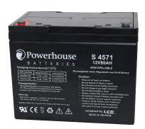
This 12V 80Ah sealed lead acid (SLA) battery is a compact battery for powering 12V equipment. It is commonly used in battery back up systems, alarm and communications systems and UPS units. Fitted with M6 bolt and nut terminals, these batteries are easily user replaced in most equipment they are used in. Cells are fully sealed to prevent any leakage of electrolyte.
