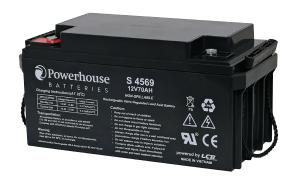
This 12V 70Ah sealed lead acid (SLA) battery is a compact battery for powering 12V equipment. It is commonly used in battery back up systems, alarm and communications systems and UPS units. Fitted with M6 bolt and nut terminals, these batteries are easily user replaced in most equipment they are used in. Cells are fully sealed to prevent any leakage of electrolyte.
