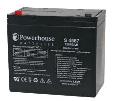
This 12V 60Ah sealed lead acid (SLA) battery is a compact battery for powering 12V equipment. It is commonly used in battery back up systems, alarm and communications systems and UPS units. Fitted with M6 bolt and nut terminals, these batteries are easily user replaced in most equipment they are used in. Cells are fully sealed to prevent any leakage of electrolyte.
