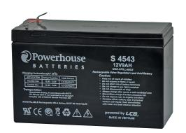
This 12V 9Ah sealed lead acid (SLA) battery is a compact battery for powering 12V equipment. It is commonly used in battery back up systems, alarm and communications systems and UPS units. Fitted with 6.3mm/F2 tab terminals, these batteries are easily user replaced in most equipment they are used in. Cells are fully sealed to prevent any leakage of electrolyte.
