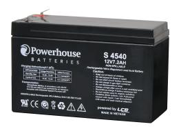
This 12V 7.2Ah sealed lead acid (SLA) battery is perhaps the most common size SLA battery in use. It is commonly used in NBN boxes, battery back up systems, alarm and communications systems and UPS units. Fitted with 4.8mm spade connection tabs, these batteries are easily user replaced in most equipment they are used in. Cells are fully sealed to prevent any leakage of electrolyte.
