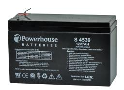
This 12V 7Ah sealed lead acid (SLA) battery is a compact battery for powering 12V equipment. It is commonly used in battery back up systems, alarm and communications systems and UPS units. Fitted with 6.3mm/F2 tab terminals, these batteries are easily user replaced in most equipment they are used in. Cells are fully sealed to prevent any leakage of electrolyte.
