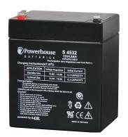
This 12V 4.5Ah sealed lead acid (SLA) battery is a compact battery for powering 12V equipment. It is commonly used in battery back up systems, alarm and communications systems and UPS units. Fitted with 4.8mm spade connection tabs, these batteries are easily user replaced in most equipment they are used in. Cells are fully sealed to prevent any leakage of electrolyte.
