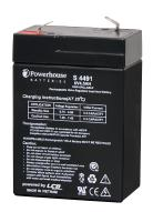
This 6V 4.5Ah sealed lead acid (SLA) battery is a compact battery for powering 6V equipment . It is commonly used in battery back up systems, alarm and communications systems and UPS units. Fitted with 4.8mm spade connection tabs, these batteries are easily user replaced in most equipment they are used in. Cells are fully sealed to prevent any leakage of electrolyte.
