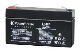
This 6V 1.3Ah sealed lead acid (SLA) battery is a compact battery for powering 6V equipment . It is commonly used in battery back up systems, alarm and communications systems and UPS units. Fitted with 4.8mm spade connection tabs, these batteries are easily user replaced in most equipment they are used in. Cells are fully sealed to prevent any leakage of electrolyte. UN Number: UN 2800 Non-Spillable - Hazard Class 8
